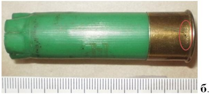
Fig. 3. Marking with an extractor: a. - general view of the extractor with a forensic marker made in a die-cut manner; б. - the result of the shooting, with the display of a ballistic code from the forensic marker on the side surface of the sleeve
