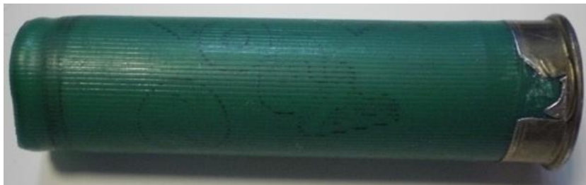
Fig. 2. Cartridge case with damage to the metal skirt when loading weapons
